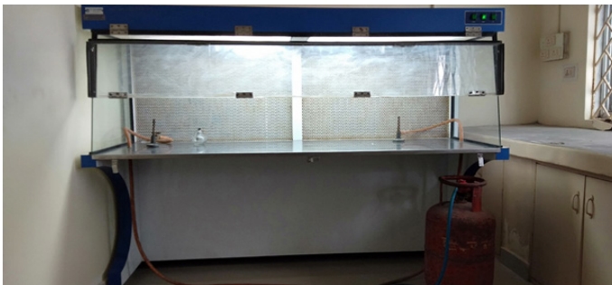
Figure 2: Laminar-air-hood with coarse filter, HEPA filter, gas cock, gas cylinder and electrical outlets
